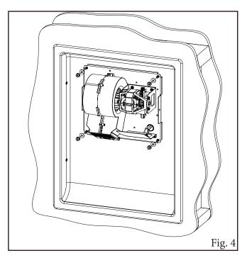
Remove the hand dryer cover and place dryer on the 4 mounting studs. Secure using (4) #10 flat washers and (4) #10-32 nuts. Connect electrical wires to dryer per the dryer schematic.
