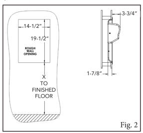
Begin with a 14-1/2" W x 19-1/2" H rough wall opening framed on all sides. Make sure the opening is the correct distance above the floor. Refer to the chart below for mounting heights.
